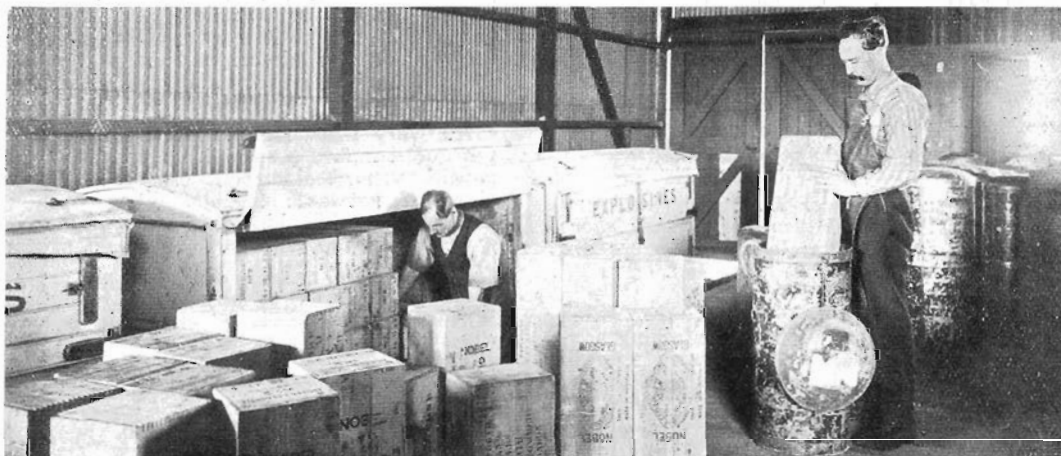
This photograph shows how the explosives are handled when they reach the Laverton railway shed. They are discharged from the Explosives' trucks on to the floor of the shed, placed in portable magazines or loaded in bulk into the powder van on the other side of the platform.
